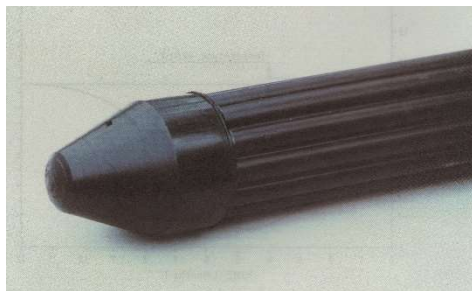
Figure 2: Coaxial BHE by SHF in Switzerland, made of PE with multi-chamber outer channel for turbulent flow and increased heat exchange (photos from Hess, 1987)
