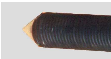
Figure 1: Coaxial BHE as tested in Schwalbach GSHP research station (Sanner, 1986), consisting of corrugated metal outer tube (usually stainless steel, but copper in this cut-out sample for exhibitions), protected against corrosion by a PE-coating (photos Sanner)
